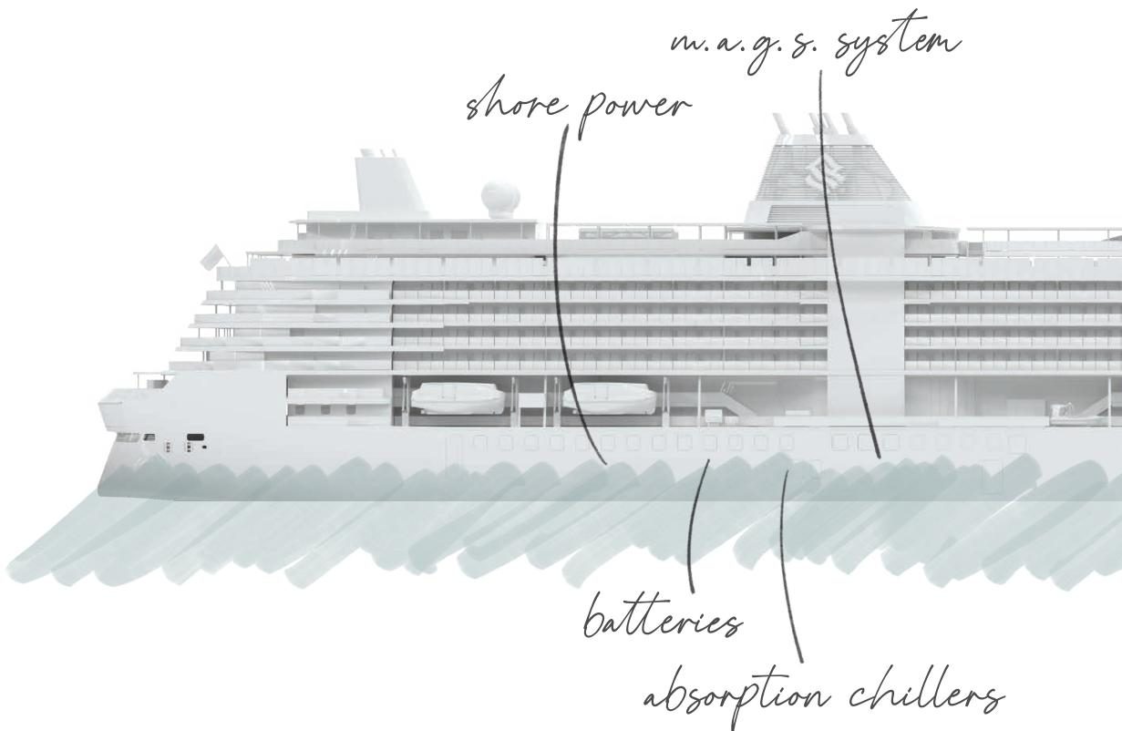
incineration emissions, and a Waste Heat Recovery System which allows the ship to reuse waste heat (ie. from the absorption chillers) for even more energy efficiency. Furthermore, she's equipped with Shore Power, a feature that allows *Silver Nova*'s main generators to be shut down and the ship plugged into the onshore energy supply where available, cutting emissions while in port.
